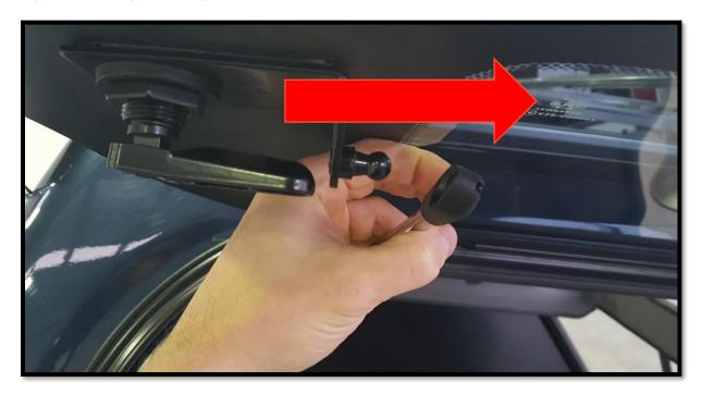
4. Lift the glass up to detach the hinge from the frame, take the glass off.
