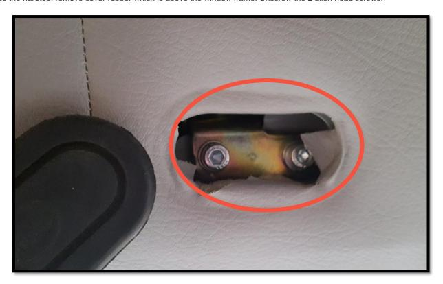
9. Take the hinge with the gas strut off the hardtop.
