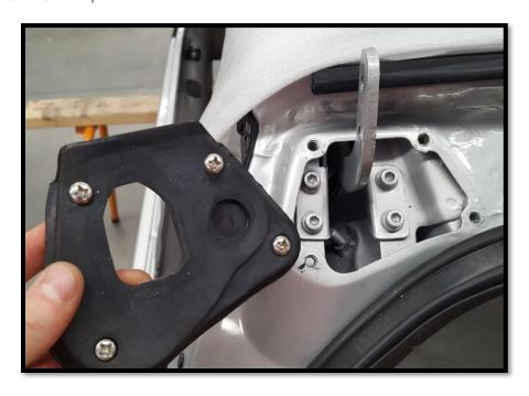
7. Remove the 4 allen head screws holding the hinge.
