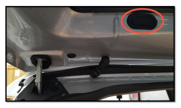
2. Pull out the wiring loom and disconnect wires. There is constant voltage so be careful and avoid the short circuit.
