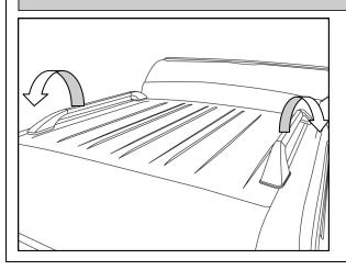
Remove the factory fitted plastic roof rails from the hardtop by unclipping the screw covers and removing the securing screws. (These will not be reinstalled)
