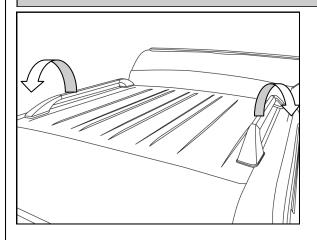
Remove the factory fitted plastic roof rails from the hardtop by unclipping the screw covers and removing the securing screws. (These will not be reinstalled)
