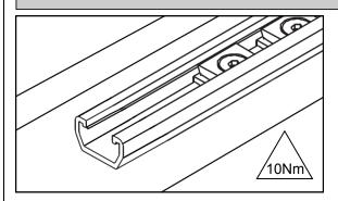
Tighten and torque up the screws to 10Nm.
